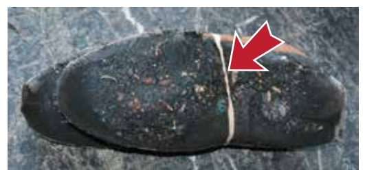
• Soles are melted, distorted and not wearable
